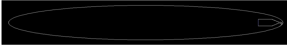
Figure 20: Elliptical cross-section airfoil with jet flap
